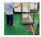
In the plant, there is a flood-proof ridge around the filament washing area. Whenever filament was washed, it needed to be transported by hand, and the cart carrying wet filament weighs 20 to 30kg, which runs the risk of causing muscular or skeletal injuries. A bridge was then built over the ridge to reduce the possibility of injuries caused by employees using force improperly to move the cart.
